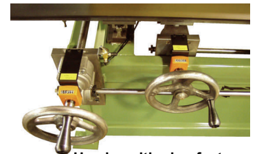
Head positioning features solid shaft coupling with digital location readouts
