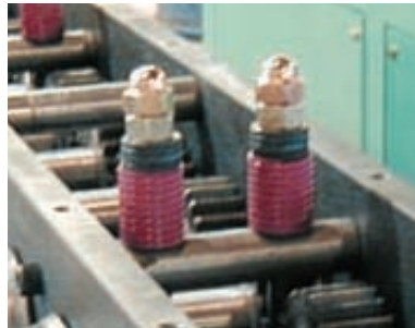
Self-Adjusting Roll Tensioner For Full Gauge Range
