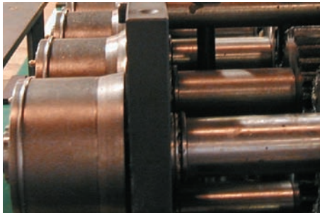
Heavy Duty anti-friction Roller & Thrust Bearings (No Bronze Thrust) All Bearings Greasable
