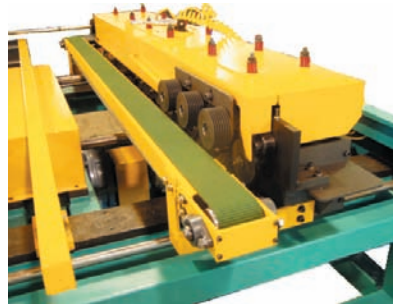
Pass Thru Conveyor's For Coil Installation
